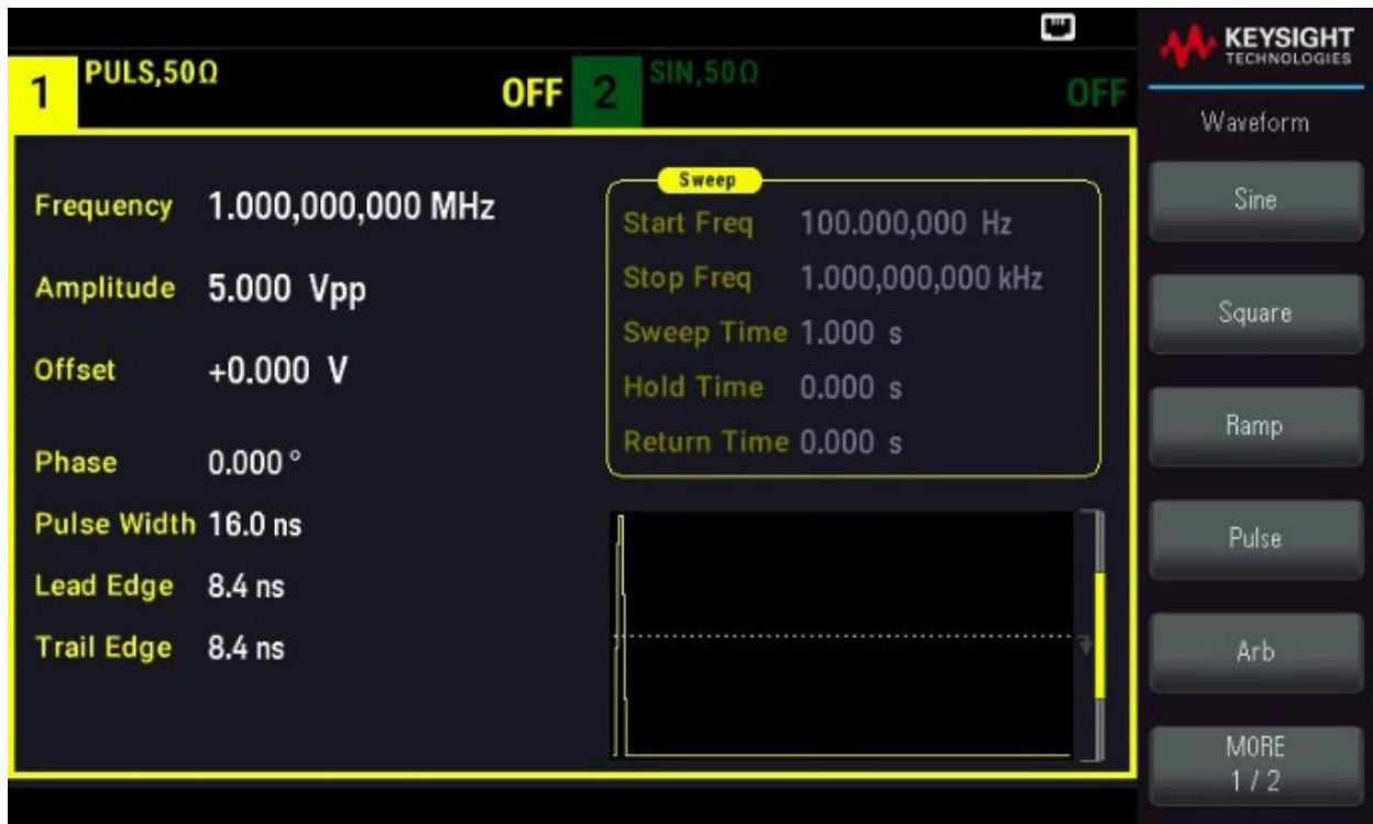
Figure 4. FG33532A function generator setting screen with the smallest possible rise and fall time of 8.4 ns.
