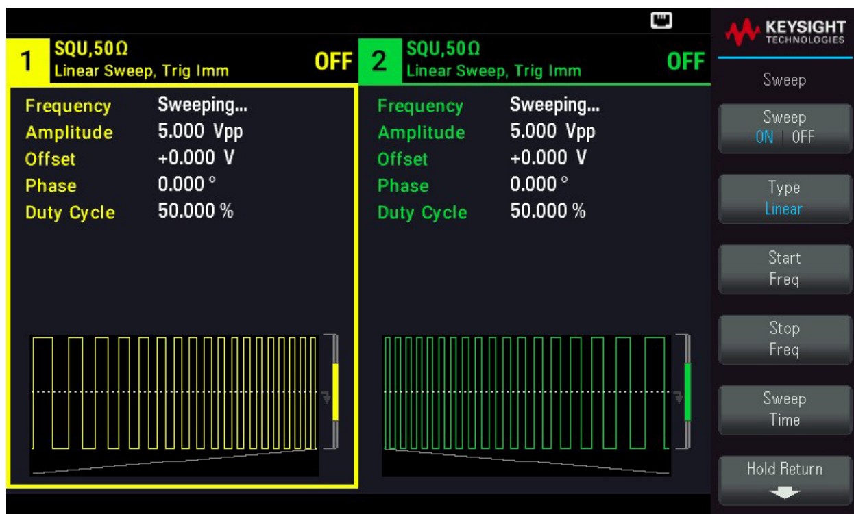
Figure 1. Performing over-frequency margining on Channel 1 and under-frequency margining on Channel 2 with the FG33532A function generator.
